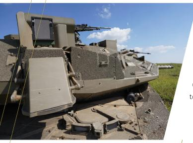
In the latest systems, the control unit also communicates with analogous systems mounted on other vehicles via the Battle Management System (BMS), so that two or more vehicles can cover each other with their active protection systems. The final component is the effector. Its purpose is to interact with the enemy's center of gravity or observation and targeting systems so as to minimize the risk of a vehicle being hit.
